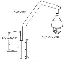
Fig. 3: Roof mount (IP66)
