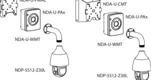
Fig. 2: Pole mount (IP66); Corner mount (IP66)
