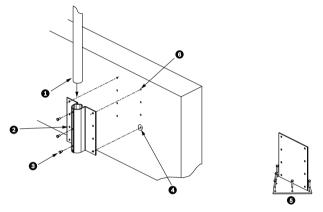
Figure 7.1: Parapet Wall Mount Bracket and Roof Mount Plate
