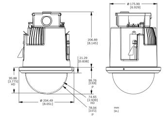
Fig. 2: AUTODOME 7000 series In-ceiling
