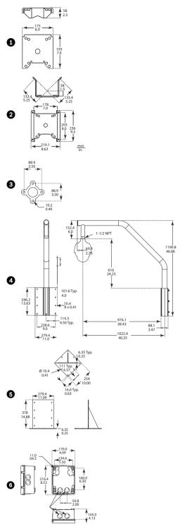
Fig. 3: AUTODOME 7000 series Optional Mounts
