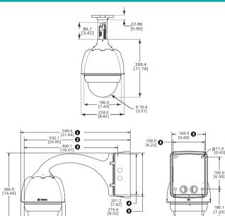
Fig. 1: Dimensions, AUTODOME7000 pipe mount, pendant mount
