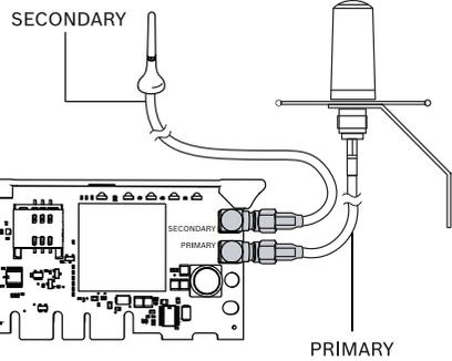
⚠ The B40 must be installed to the Primary connector.
