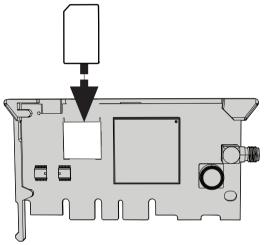
Figure 3.1: Inserting the SIM card
