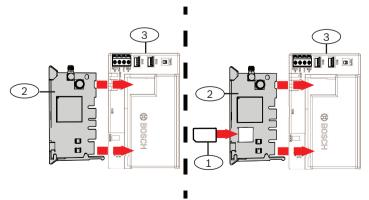
Figure 3.6: Communicator installation (B450 shown)
