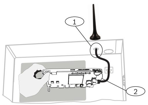
Figure 3.2: Installing the antenna
