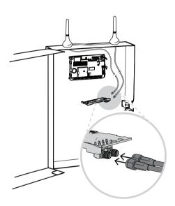
Figure 3.4: B444-A/B444-V cable connection
