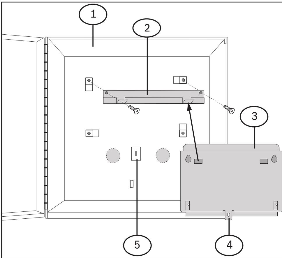
Figure 1: D6103 Enclosure and L901 mounting bracket
