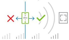
RSSI values can vary greatly depending on many factors, including the type of transmitting device, battery-level, and the material and thickness of nearby walls. There is no linear relation between the RSSI value and distance between transmitter and receiver.
