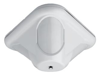
The ceiling mount DS939 PIR Detectors provide up to 16.4 m (54 ft) panoramic coverage pattern and can be mounted on ceilings as high as 6.1 m (20 ft). With three separate PIR sections that are fully adjustable, the DS939 detectors provide coverage integrity at all mounting heights, plus the ability to customize the coverage for specific areas. The DS939 detectors use several processing techniques to provide excellent catch performance with freedom from false alarms.
