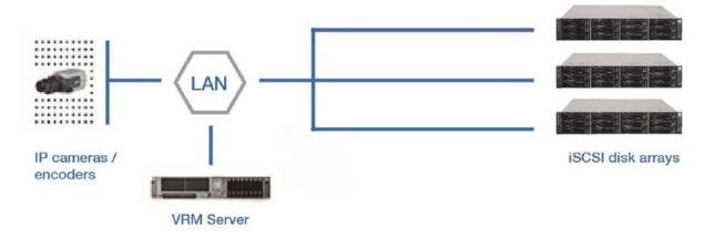
Figure 9 shows a large-scale VRM architecture.
