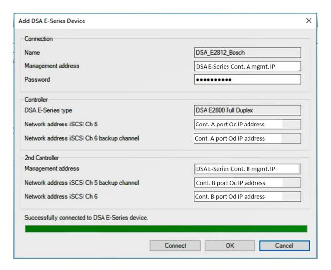
**Note:** In this example, the primary recording ports are controller A port 0c (port 5 from Figure 7) and controller B port 0d (port 6 from Figure 7). Controller B port 0c and controller A port 0d are the backup ports for the primary recording paths.
