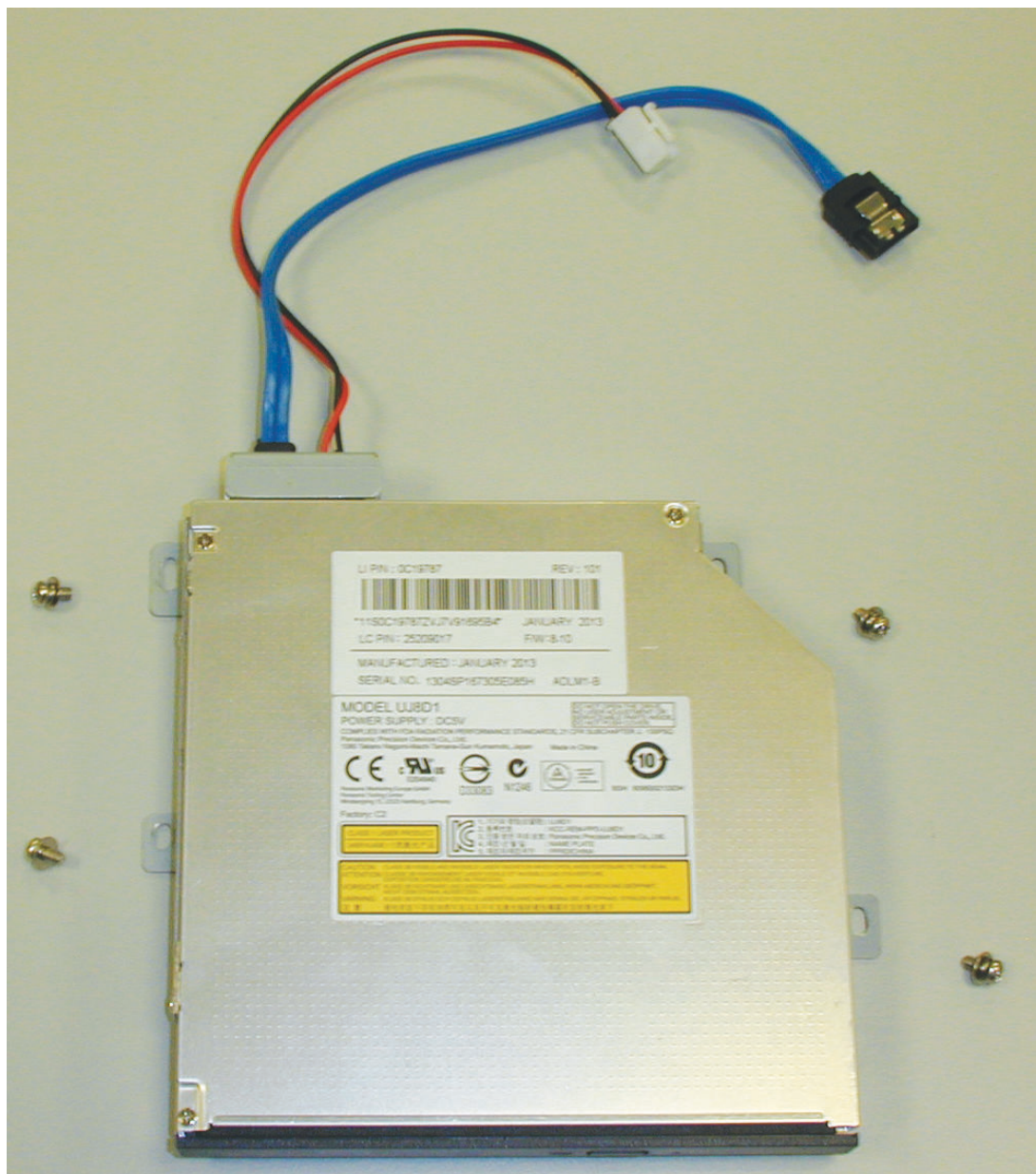
Figure 5.7: DVD install components for DIVAR AN 3000
