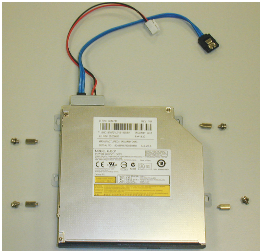
Figure 5.9: DVD install components for DIVAR AN 5000
