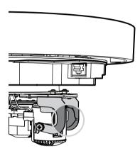
3. Do not tilt each of the four lenses any further than until the white dot on the edge of the lens holder meets the white triangle. If you tilt any further, you might see a partly blurry image. Use this position only in specific use cases or when you need the lens to fully zoom in.
