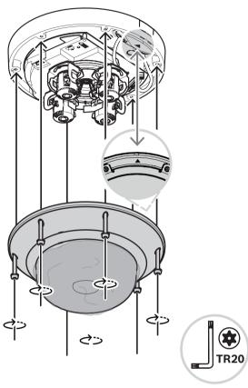
3. Remove the protective cover from the bubble.
