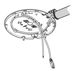
10. Install the conduit cover on the conduit plate with the bolt. Tighten the screw between 1.4 and 2 Nm (1 lbfft and 1.5 lbfft) with the TR20 Allen key.
