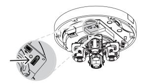
3. Re-attach the camera dome cover onto the camera base.
