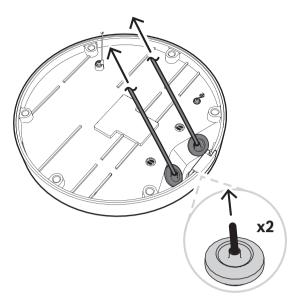
12. If required, do a loop with the cable on the hooks of the mounting plate.
