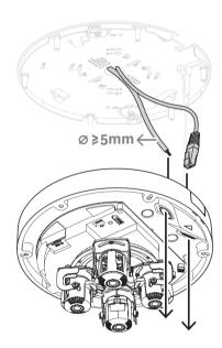
11. Fix the M20 rubber grommets in both cable inlets to make sure that the cable inlets are firmly closed.
