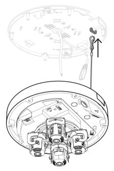
Put the RJ-45 punch-through aid on the network cable.
