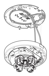
13. Position the camera base on the mounting plate, so that the screw holes of camera base and mounting plate match. Slightly press the camera base onto the mounting plate until you hear/feel a click. Make sure that the camera base is secured.
