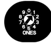
The B426 has specific rotary switch settings for SDI Addresses 88 and 92 or SDI2 Addresses 1 and 2 when used to communicate with Remote Programming Software (RPS) or with a central station network receiver. Refer to *Table 28* for the correct switch settings. When the Reset Pin (labeled S1) is closed, all SDI communication module addresses are automatically enabled for RPS communication without restriction.
