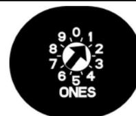
The B420 has specific rotary switch settings for SDI Addresses 88 and 92 or SDI2 Addresses 1 and 2 when used to communicate with Remote Programming Software (RPS) or with a central station network receiver. Refer to *Table 29* for the correct switch settings. When the Reset Pin (labeled S1) is closed, all SDI communication module addresses are automatically enabled for RPS communication without restriction.
