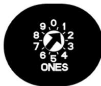
The B450 has specific rotary switch settings for SDI addresses 88 and 92 or SDI2 addresses 1 and 2 when used to communicate with Remote Programming Software (RPS) or with a central station network receiver. Refer to *Table 27* for correct switch settings.
