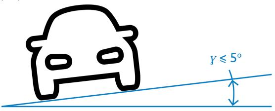
For best performance the tilt angle should be within the range of  $-5^{\circ} \le \gamma \le +5^{\circ}$ , but must be within the range  $-30^{\circ} \le \gamma \le +30^{\circ}$ .
