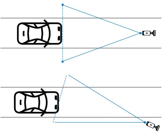
The field of view should be at least twice as wide as the lane to ensure that the front of the vehicle is visible.
