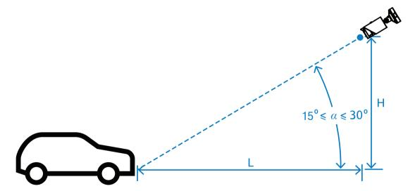
The installation height H depends on the availability of mounting constructions, and in practice this means:
