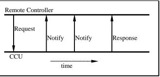
Figure 2 Message flow during a Remote function
