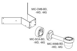
Typical Corner mount configuration Not shown: Mounting hardware.
