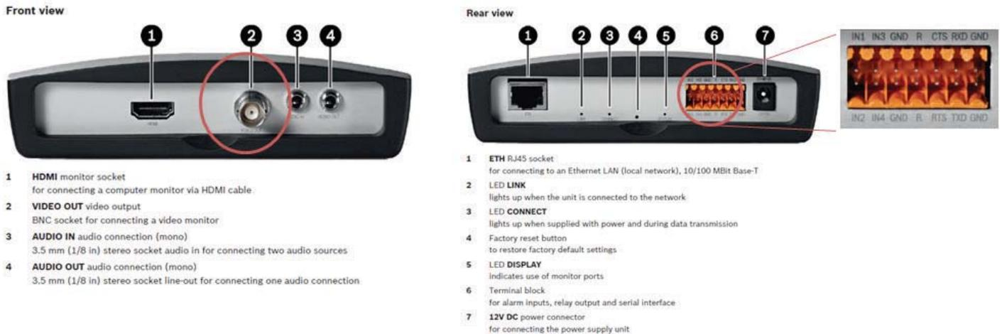
Figure 15: Interface ports for integration with monitoring and control equipment.
