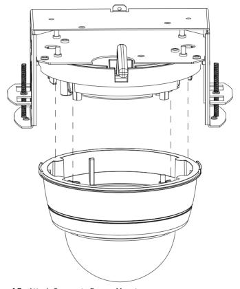
Figure 4.7 Attach Camera to Recess Mount
