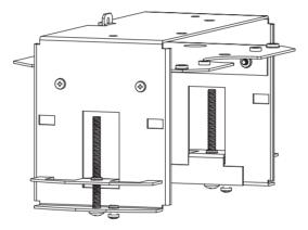
Figure 4.4 Attach Recess Mount to Ceiling
