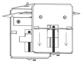
Figure 4.3 Attach Recess Mount to Ceiling
