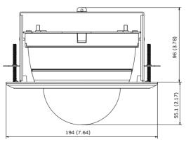
Figure 4.1 Recess Mount Dimensions
