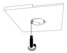
Figure 4.5 Tighten Mounting Clamps
