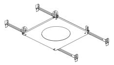
Figure 4.2 Mounting bracket
