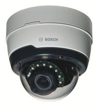
The FLEXIDOME IP 3000i IR is built for high quality, 24/7 performance, with a range of reliable surveillance features, including Essential Video Analytics, and is designed for easy installation. The built-in active infrared illuminator provides high performance in extreme low-light environments. The camera is for outdoor use and has a resolution of 5 MP.
