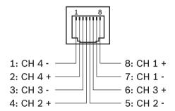
Figure 6.4: Pin assignment of the LINE OUT 1-4 socket
