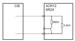
Figure 6.13: Internal configuration of the REL contact (VDE 0833-4)
