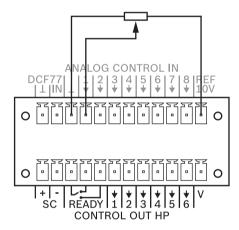
Figure 6.10: Sample application of a control input and use of an analog input signal
