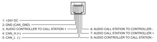
Figure 6.5: Pin assignment of CST BUS port
