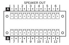
100 V or 70 V loudspeakers can be connected on each speaker output with the 2 (two) 12-pin connectors that are delivered with the device. Loudspeaker cables with a cross sectional area from 0.14 mm<sup>2</sup> (AWG26) up to 1.5 mm<sup>2</sup> can be used.
