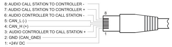
Figure 6.6: Pin assignment of CST BUS connector
