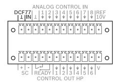
The top half of the control port has an input for the radio receiver of the DCF77 signal. Observe the delivered documentation when connecting a 3<sup>rd</sup> party DCF receiver to the controller.
