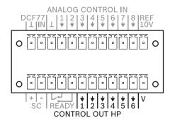
The lower half of the control port has six freely programmable **h**igh **p**ower (HP) control outputs numbered 1 through 6. In inactive mode (Off), these control outputs are open, while in active mode (On), they are closed to ground. To operate the externally connected elements, a voltage source is available on the connection V; see also the following diagram.
