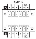
The AMP IN audio inputs allow to connect the 100 V (or 70 V) output signals of two 2-channel power amplifiers (up to four power amplifier channels) to the integrated 2-in-6 router blocks A or B. Additionally there are two input channels for spare amplifiers.
