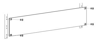
Figure 5.1: Installation of the device into a 19" rack
