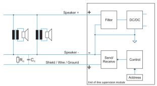
Figure 8.1: Circuit diagram (R<sub>G</sub> and C<sub>G</sub> are caused by the loudspeaker installation, e.g. wire type, length)
