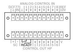
The lower half of the control port has a potential-free READY changeover contact. This changeover contact signals to other devices that the controller is ready for operation or indicates faults in the system. The following table shows the possible statuses of the ready contact.
