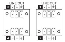
The audio outputs are electronically balanced. You must always use a balanced audio signal at the output of the device where this is possible. The scope of delivery for the device includes 3-pin connectors. Conductor cross-sections of 0.14 mm<sup>2</sup> (AWG26) to 1.5 mm<sup>2</sup> (AWG16) can be used.
