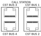
The four **C**all **ST**ation (CST) BUS ports connect call stations with the controller. This are 8-pole RJ-45 ports that integrate the power supply, control interface (CAN bus), and audio interface. Every CST BUS supports up to 4 call stations. In total 16 call stations can be connected to one controller.
