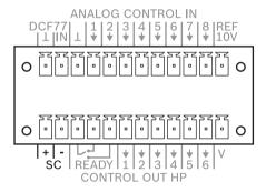
The lower half of the control port has a special, short-circuit-proof output for polarity switch impulses. Slave clocks connected here are automatically adjusted if a time difference is detected between the slave clocks and the system clock, for example after a power failure or in the event of manual input. Ensure that all slave clocks are connected with the same polarity. Recommended connecting cable: shielded flexible stranded wire, LiY, 0.5 mm<sup>2</sup>.
