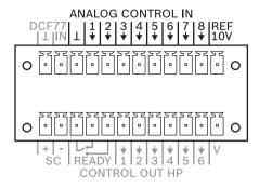
The upper half of the control port has eight freely programmable control inputs for voltages of between 0 volts and 10 volts. The inputs are numbered 1 through 8. The controller provides its own voltage supply for externally connected control elements, e.g., a potentiometer. The voltage supply is available at the control port connections for 10V REF and ground; see the following diagram.
