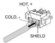
Figure 6.1: Balanced cabling
