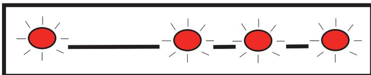
Figure 2.1: Firmware version LED pattern (v1.3 shown)
