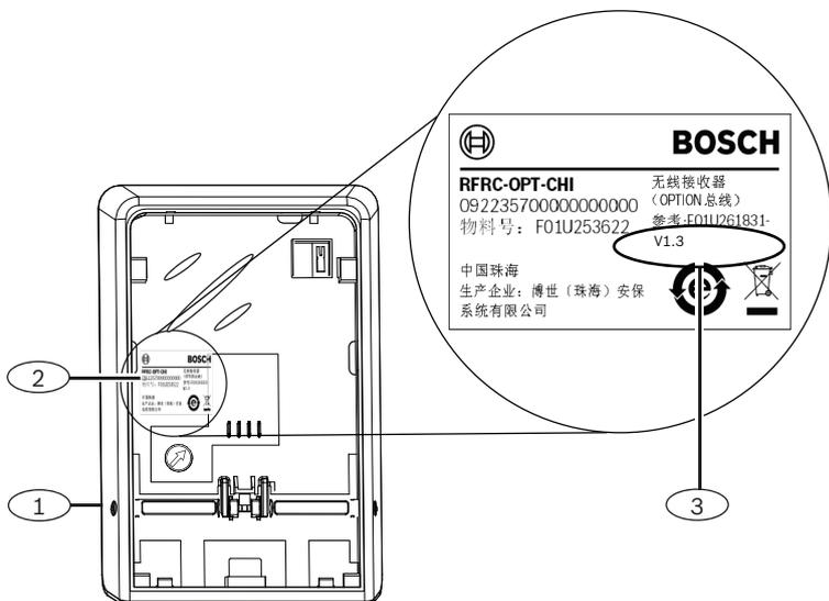
**Figure 2.3: RFRC-OPT-CHI receiver label and firmware version**
