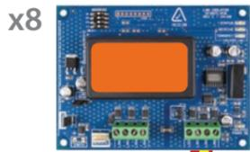
Up to 8 LAN Isolator modules can be connected. Isolators provide electrical isolation between LAN segments reducing the chance of surge damage. Isolators can also be used to increase the total LAN length beyond 1200m.
