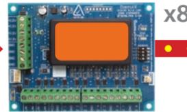
Up to 8 zone expanders of any type can be connected to the system. When using Single or Alarm & Tamper EOL, the CM707B can be installed to provide 16 zones on the CM705B Expander. The CM707B cannot be installed when using split EOL monitoring.
