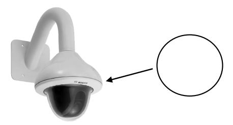
In certain installations in humid environments, moisture can enter the FLEXIDOME Wall Mount. This causes condensation on the inside of the camera's bubble. To prevent this, a rubber gasket\* is added to the VDA-WMT-DOME - FLEXIDOME Wall Mount. It is recommended to use this rubber gasket in certain outdoor installations or installations in humid environments.
