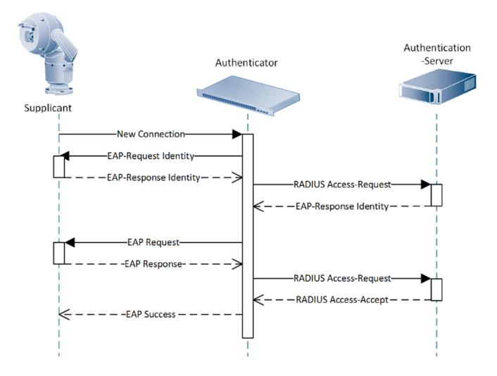
Figure 2: 802.1x Authentication Sequence Diagram
