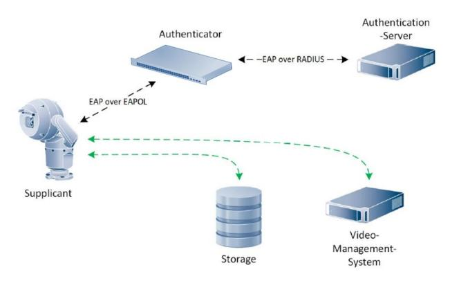
Figure 1: EAP (Extensible Authentication Protocol) data is first encapsulated in EAPOL frames between the Supplicant and Authenticator, then re-encapsulated between the Authenticator and the Authentication Server using RADIUS or Diameter.
